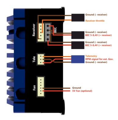
Usually in helicopters, the receiver- and BEC-cables will be wired from the front to the rear alongside the motor. Make sure that the receiver-, tele- and BEC-cables have to be wired together on one side!
