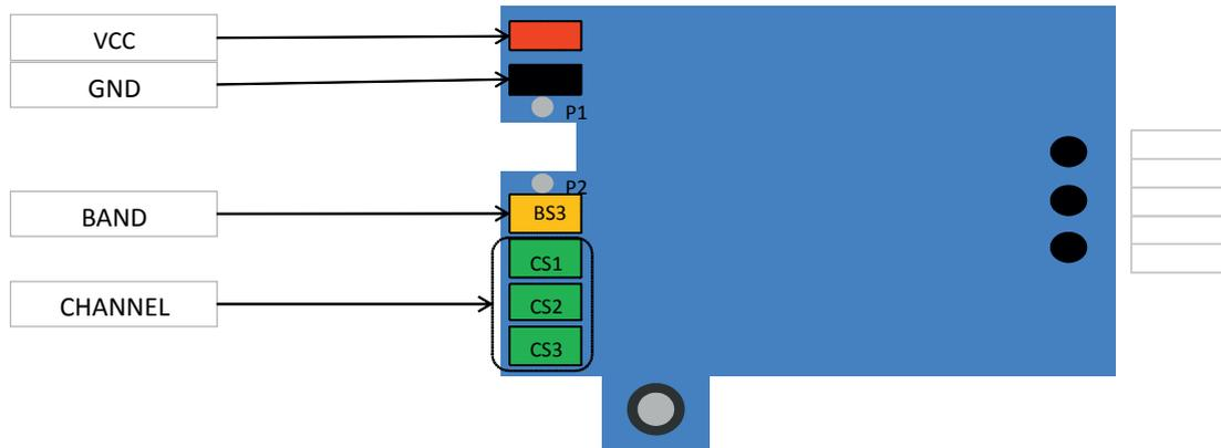
VCC connected to 4.5...5V
