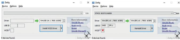
To Flash the Firmware you have to enter the so called DFU mode. On Windows 10 I had to use a tool called Zadig (download and start it) to be able to switch drivers for DFU mode to work. In order to switch drivers you have to take the following steps.
