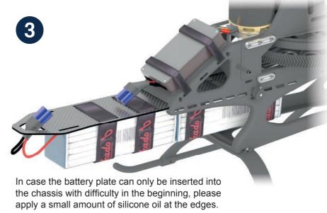
Before each flight make sure that the battery plate is secured with both quick release mechanisms.
