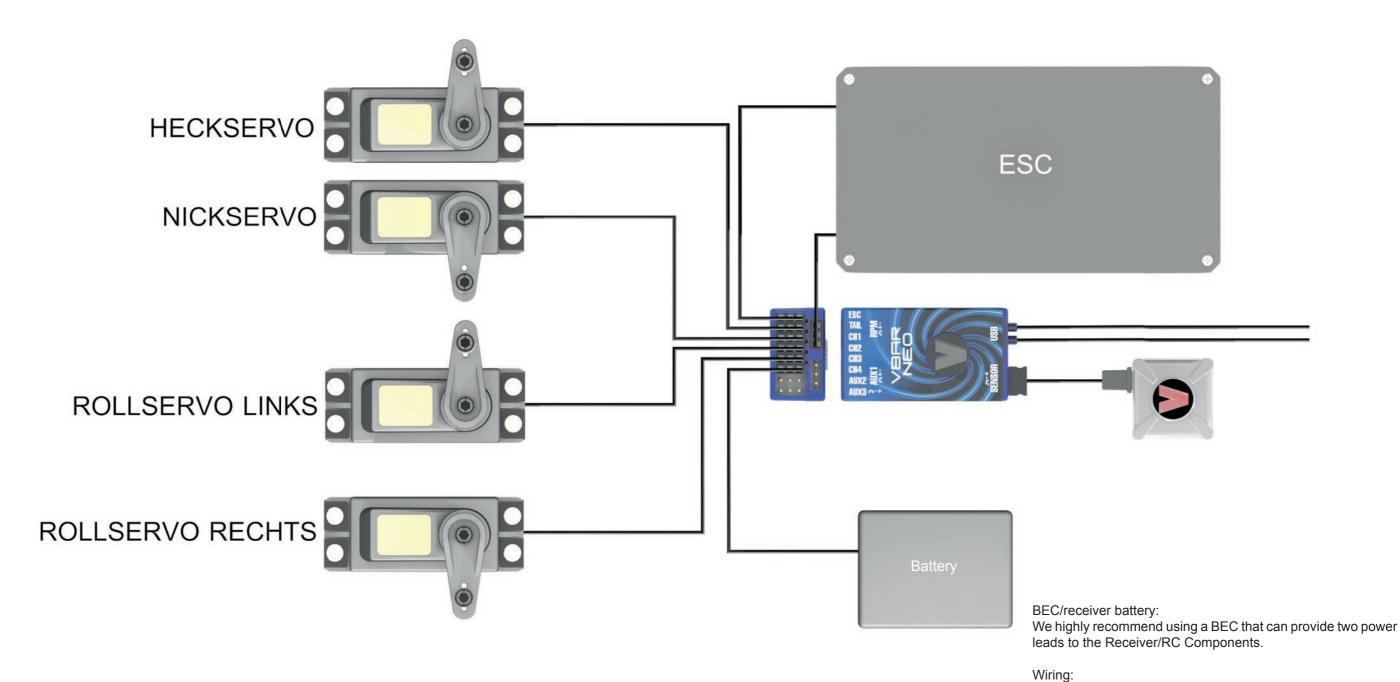
Please note: All wires must be placed in such a way that they cannot be damaged by any sharp edges during operation of the helicopter. Please apply the fabric tube and the edge guard provided in this kit. Both types of protection are also available individually from Mikado.
