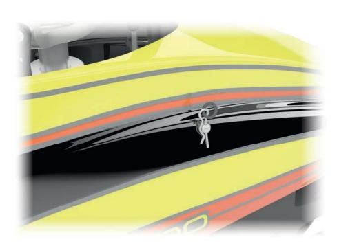
The canopy of the LOGO 700 is mounted via four attachment points. The two attachment points in the front ensure that the canopy sits well on the chassis during flight. have a guiding function. In the back, the canopy is attached by two rubber grommets. You will find another, high-quality, set of rubber grommets included in the kit. You may use these, if desired.
