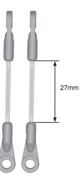
Note when mounting the ball links: One side of the ball link will clip on easily. The other one is too tight to clip on easily. The brand name Gabriel must point outwards.
