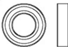
Bearing 軸承 (φ 12x φ 24x6mm) x 3
