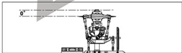
Stick position at middle/Throttle 90%/Pitch 0° 搖桿中速/油門90%/Pitch 0°
