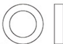
Bearing 軸承 ( \phi 12x \phi 18x4mm ) x 2
