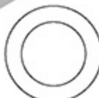
Bearing 軸承 ( \phi 12x \phi 18x4mm ) x 2
