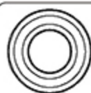
Bearing 軸承 (φ8xφ16x5mm) x 2
