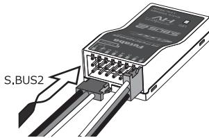
Plug the temperature sensor into the S.BUS2 output of your telemetry receiver, either directly or via a Y-lead or HUB lead.
