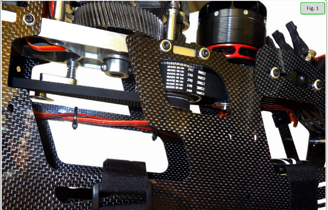
Figure 1: Shows the wiring which connects the receiver and ESC . If the BEC used is combined with the ESC, it is recommended to use a dual wire connection.
