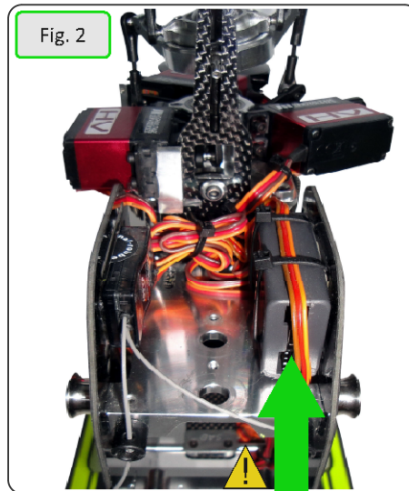
It is important to lock the plugs of the flybarless unit with an adhesive - for example hot glue.
