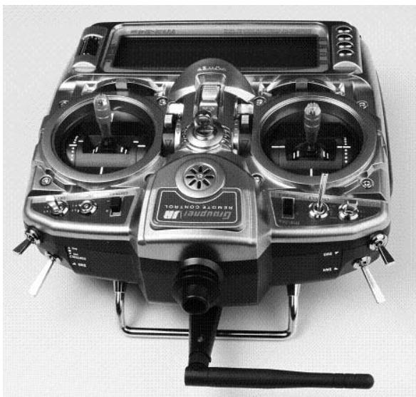
For applications where the model is not operated directly above or below the transmitter, the optimum aerial orientation is vertically upwards; this applies in particular to model cars and boats:
