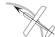
Nose Points inside circle Too much coupling or differential. Reduce one or both.
