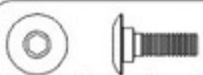
Socket button head collar screw 半圓頭內六角輪套螺絲 (M3x8mm) x 4
