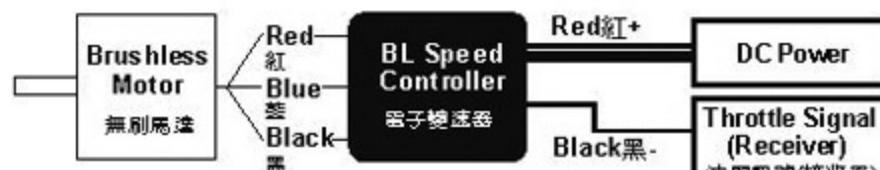
The motor rotates in different direction with different brand ESCs. If the wrong rotating direction happens, please switch any two cables to make the motor rotates in right direction.
